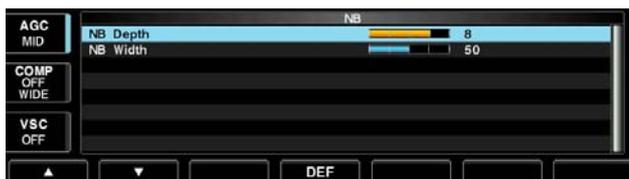
To deal with various type of noise, attenuation level and noise blanking duration can be set in NB set mode.
