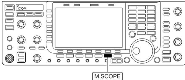
The mini scope screen can be displayed with another screen display, such as set mode menu, decode screen, memory list screen, etc. simultaneously.
