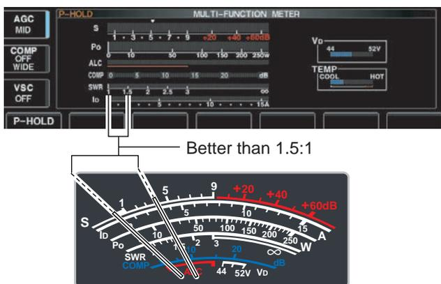
The SWR meter indicates the SWR over the transmission line in all modes.
