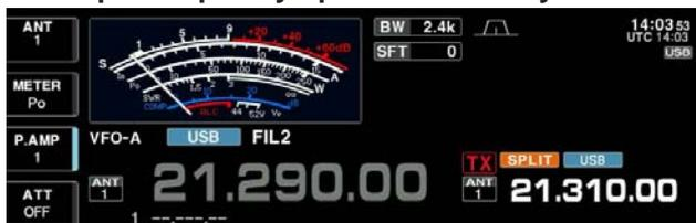
Split frequency operation allows you to transmit and receive in the same mode on two different frequencies. Split frequency operation is performed using 2 frequencies on the main and sub readouts.
