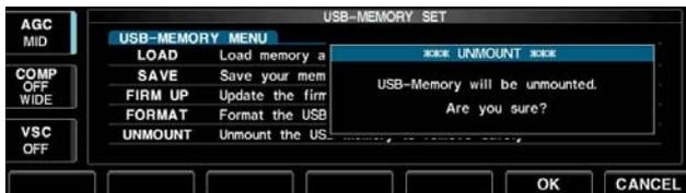
**CAUTION!** When removing the USB-Memory, unmount operation is recommended. If you do not unmount the memory in this case, data in the USB memory may be corrupted.
