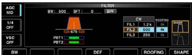
▨ The filter set screen graphically displays the CW pitch operations. (See at left.)
