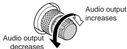
**23 RF GAIN CONTROL [RF]** (outer control; p. 3-9)
