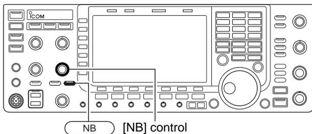
The noise blanker eliminates pulse-type noise such as the noise from car ignitions. The noise blanker is not available for FM mode.
