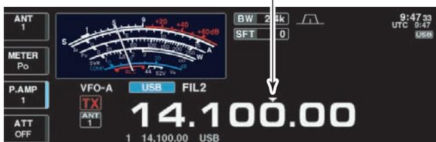
The operating frequency can be changed in larger steps (0.1, 1, 5, 9, 10, 12.5, 20 or 25 kHz selectable) for quick tuning.
