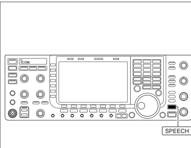
The IC-7700 has a built-in voice synthesizer to announce the frequency, mode, etc. (S-meter level can also be announced—p. 12-15) in clear, electronically-generated voice, in English (or Japanese).
