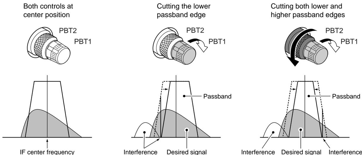
PBT (Passband Tuning) electronically narrows the IF passband width by shifting the IF frequency slightly outside of the IF filter passband to reject interference. The IC-7700 uses DSP for the PBT function. Moving both [TWIN-PBT] controls to the same position shifts the IF both above and below the received frequency.
