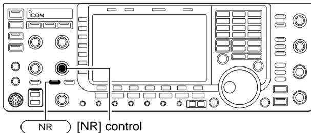
The noise reduction function reduces random noise components and enhances desired signals which are buried in noise. The DSP performs the random noise reduction function.
