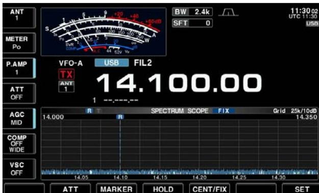
Displays signals within the specified frequency range. Conditions on the selected frequency band can be observed at a glance when using this mode.
