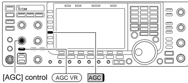
The AGC (auto gain control) controls receiver gain to produce a constant audio output level even when the received signal strength varies greatly.
