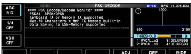
Adjust the PSK decoder threshold level if some characters are displayed when no signal is received.
