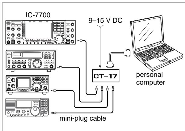
The transceiver can be connected through an optional CT-17 CI-V LEVEL CONVERTER to a PC equipped with an RS-232C port. The Icom Communications Interface-V (CI-V) controls the transceiver.
