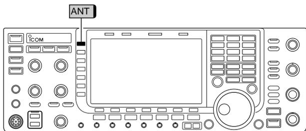
The IC-7700 has 4 antenna connectors for the HF/50 MHz bands, [ANT1], [ANT2], [ANT3], and [ANT4].
