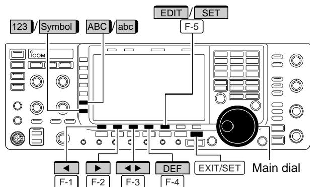
The IC-7700 has a built-in calendar and 24-hour clock (accuracy  $\pm 75$  sec. per month) with daily power ON/OFF timer functions. Before operating these timer functions, set the current date and time.
