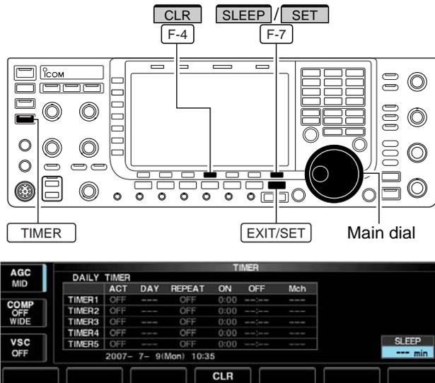
The sleep timer turns the transceiver power OFF automatically after passing the set period. The timer can be set to 5–120 min. in 5 min. steps.
