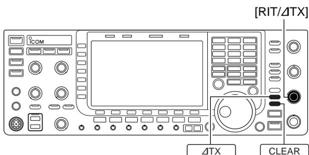
The ΔTX function shifts the transmit frequency up to ±9.999 kHz in 1 Hz steps (10 Hz steps when cancelling the 1 Hz step readout) without moving the receive frequency.
