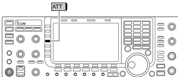
The attenuator prevents a desired signal from distortion when very strong signals are near the desired frequency or when very strong electromagnetic fields, such as from broadcast stations near your location.
