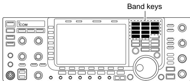
The triple band stacking register provides 3 memories for each band key, storing frequency and mode information.
