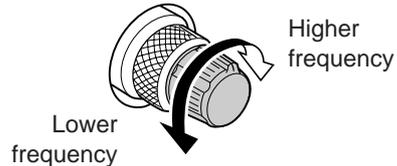
**65 MANUAL NOTCH FILTER CONTROL [NOTCH]**
