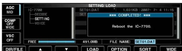
By loading the saved setting file from the USB-Memory, you can easily set up another IC-7700—several operators settings can easily be applied to one IC-7700.
