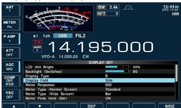
2 types of screen images and 5 types of frequency readout indication fonts are available in the IC-7700.
