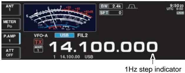
A minimum tuning step of 1 Hz can be used for fine tuning.
