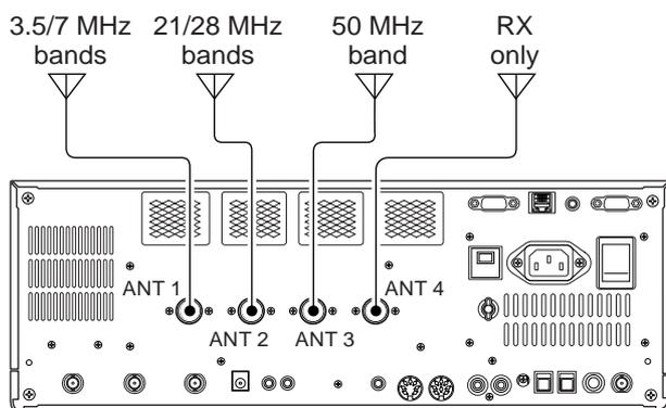
After an antenna has been selected for use (by pushing [ANT] (MF1)), the antenna is automatically selected whenever that band is used.
