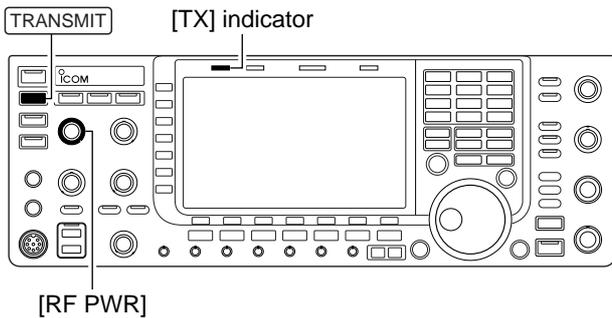
Before transmitting, monitor your selected operating frequency to make sure transmitting won't cause interference to other stations on the same frequency.
