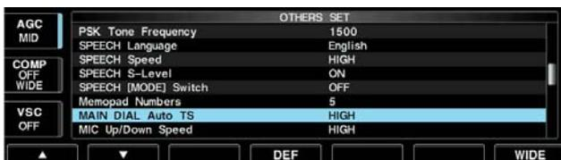
When rotating the main dial rapidly, the tuning speed accelerates automatically as selected.
