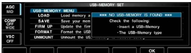
**NOTE:** If no USB-Memory is inserted and [FORMAT] [F-4] is selected as in step ①, an error message appears.
