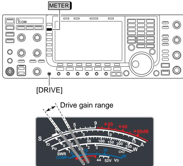
The drive gain is active for all modes other than SSB mode with speech compressor OFF. The [DRIVE] control adjusts the gain of the driver stage.
