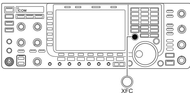
When the ΔTX function is ON, pushing and holding [XFC] allows you to monitor the operating frequency directly (ΔTX is temporarily cancelled).
