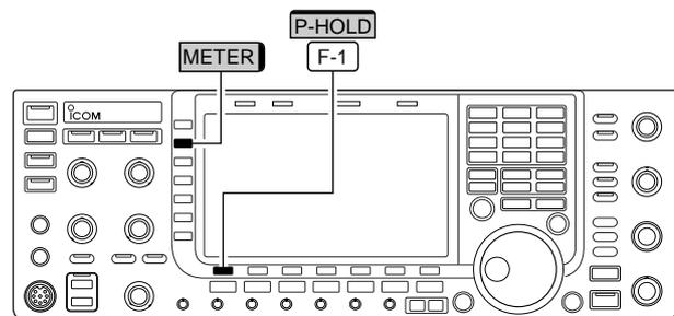
The IC-7700 can display the multi-function digital meter on the LCD display. This meter displays all transmit parameters simultaneously.
