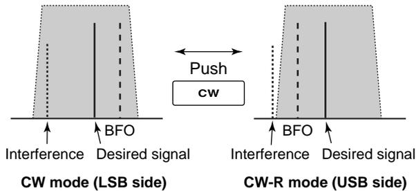
CW-R (CW Reverse) mode uses the opposite side band to receive CW signals.
