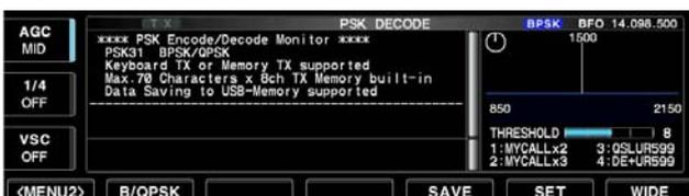
• PSK decode screen— QPSK mode
