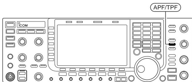
The twin peak filter changes audio frequency response by boosting the mark and space frequencies (2125 and 2295 Hz) for better reception of RTTY signals.
