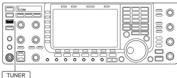
The internal automatic antenna tuner matches the transceiver to the connected antenna automatically. After the tuner matches an antenna, the variable capacitor settings are memorized as a preset point for each frequency range (100 kHz steps). Therefore, when you change the frequency range, the variable capacitors are automatically preset to the memorized setting.
