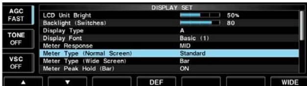
A total of 3 meter types are available in the IC-7700—Standard, Edgewise and Bar meters. Follow the instructions below for the meter type selection.
