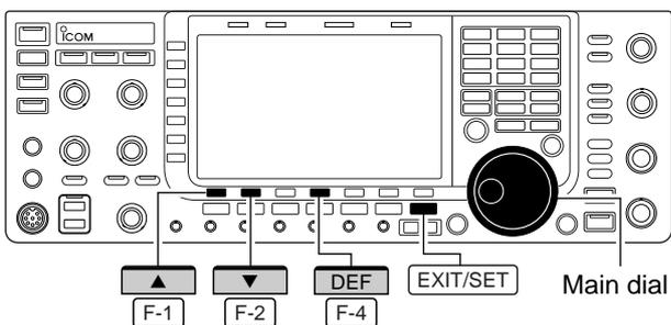
When the squelch is open, scan continues until it is stopped manually—it does not pause on detected signals. When squelch is closed, scan stops when detecting a signal, then resumes according to the scan resume condition. Scan speed and the scan resume condition can be set using the scan set mode.
