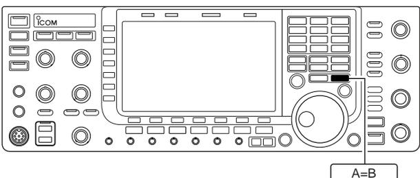
➔ In VFO mode, push and hold **A=B** for 1 sec. to set the undisplayed VFO frequency and mode to those of the displayed VFO.
