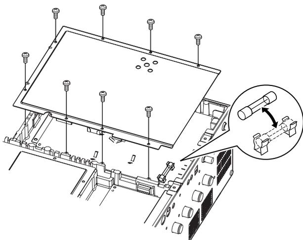
When no external DC output is available from [EXT DC] and ACC connectors, the internal fuse may be open. Replace the fuse in this case.
