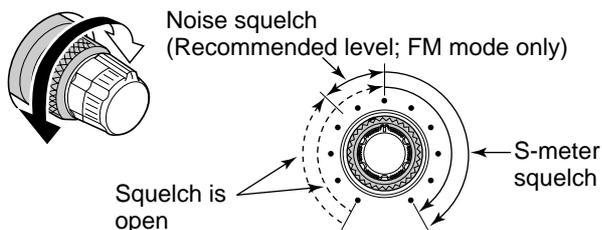
The squelch mutes noise output from the speaker (closed squelch) when no signal is received.
