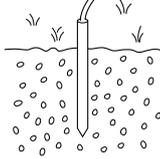
Use the heaviest gauge wire or strap available and make the connection as short as possible.
