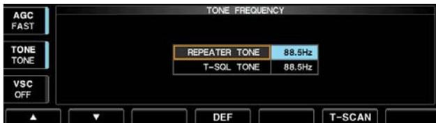
Some repeaters require subaudible tones to be accessed. Subaudible tones are superimposed on your normal signal and must be set in advance. The transceiver has 50 tones from 67.0 Hz to 254.1 Hz.
