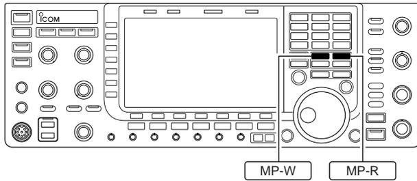
The transceiver has a memo pad function to store frequency and operating mode for easy write and recall. The memo pads are separate from memory channels.
