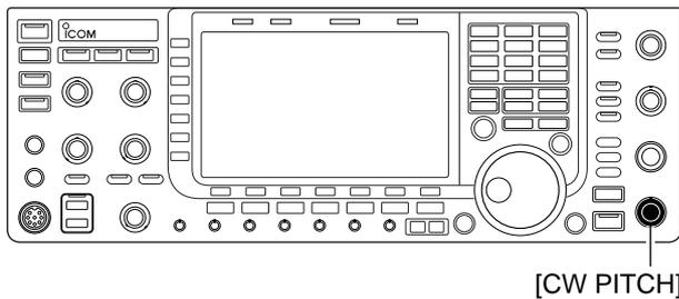
The received CW audio pitch and CW side tone can be adjusted to suit your preference (from 300 to 900 Hz in 5 Hz steps). This does not change the operating frequency.
