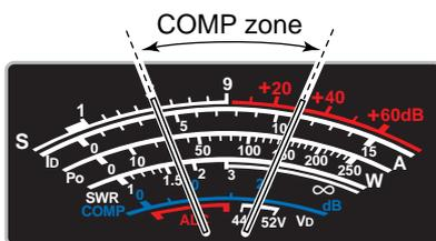
① Select USB or LSB mode and adjust [MIC] to a suitable level.
