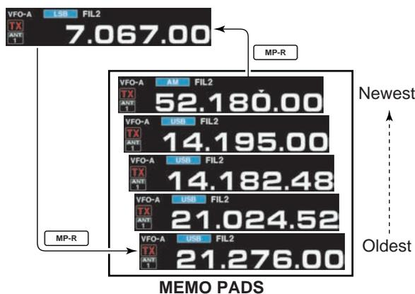
You can call up the desired frequency and operating mode of a memo pad by pushing **[MP-R]** several times.
