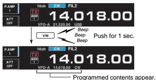
The frequency and operating mode in a memory channel can be transferred to the VFO. Frequency transfers can be performed in either VFO mode or memory mode.
