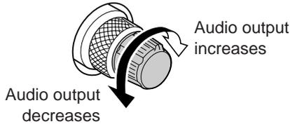
➤ Rotate [AF] control clockwise to increase, counterclockwise to decrease the audio output level.
