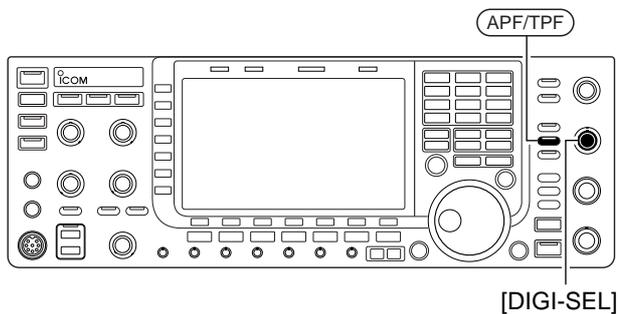
The APF changes the audio frequency response by boosting a particular frequency to enhance a desired CW signal.
