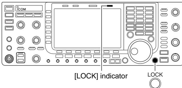
The dial lock function prevents frequency changes by accidental movement of the tuning dial. The lock function electronically locks the dial.
