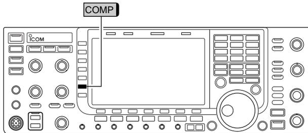
➔ During USB or LSB mode selection, push and hold [COMP] (MF6) for 1 sec. several times to select the desired transmit filter width from wide, middle and narrow.
