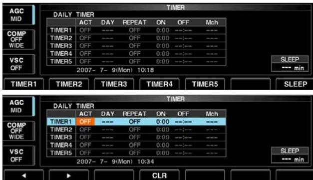
The transceiver turns power ON and/or OFF automatically on the specified day and time, with the specified frequency settings.
