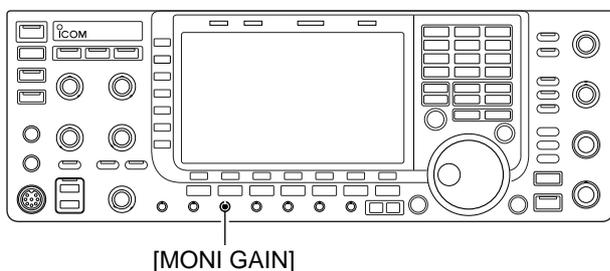
When the transceiver is in receive (and the break-in function is OFF— p. 6-3) you can listen to the CW side tone without actually transmitting.
