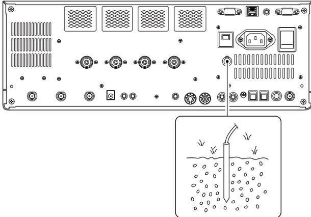
To prevent electrical shock, television interference (TVI), broadcast interference (BCI) and other problems, ground the transceiver through the GROUND terminal on the rear panel.
