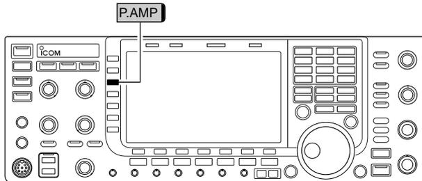
The preamp amplifies received signals in the receiver front end, to improve the S/N ratio and sensitivity. Set this to preamp 1 or preamp 2 when receiving weak signals.
