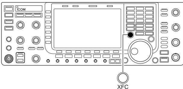
When the RIT function is ON, pushing and holding **[XFC]** allows you to monitor the operating frequency directly (RIT is temporarily cancelled).
