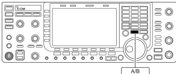
➔ In VFO mode, push **A/B** to toggle VFO-A and VFO-B.
