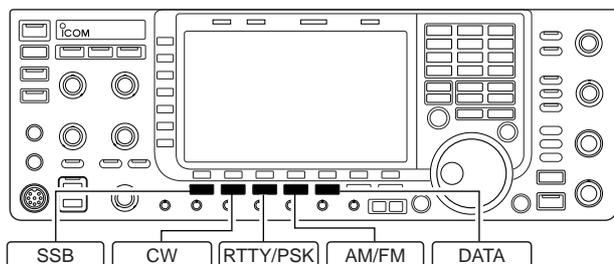
SSB (USB/LSB), SSB data (USB data/LSB data), CW, CW reverse (CW-R), RTTY, RTTY reverse (RTTY-R), PSK, PSK reverse (PSK-R), AM, AM data, FM and FM data modes are available in the IC-7700. Select the desired operation mode as follows.
