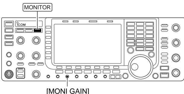
The monitor function allows you to monitor your transmit IF signals in any mode. Use this to check voice characteristics while adjusting SSB transmit parameter (p. 12-5). The CW sidetone functions regardless of the **[MONITOR]** switch setting.
