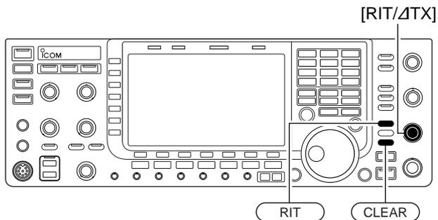
The RIT (Receive Increment Tuning) function compensates for off-frequency operation of the received station.
